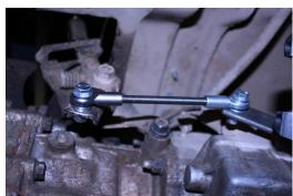
New rod installed, test shift to make sure the rod is adjusted correctly, jam nuts should be used against the rod ends to avoid the all thread from backing out.
