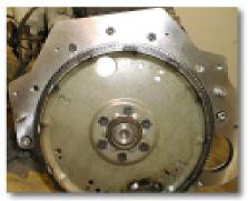
Install the flexplate to the engine crank using the proper bolts and torque specifications. Make sure the flexplate has clearance and does not drag on adapter plate.
