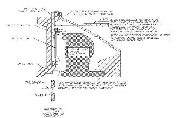
When replacing a manual transmission with a GM automatic transmission, you will need new shorter crank bolts to mount the new flexplate to your engine. These bolts can be obtained at your Jeep dealer under Part No. J3151407. Along with these bolts, Jeep also used a bolt ring on the flexplate to strengthen the bolting surface. This ring is Jeep Part No. J3214094.
