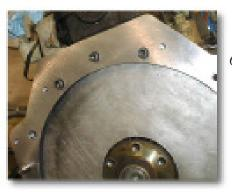
5. Insert the 5 allen head cap screws into the engine or dust sheild. **DO NOT TIGHTEN ANY BOLTS UNTIL ALL 3 BOLTS HAVE BEEN STARTED AND SNUGGED UP.** Torque to 30 ft./lbs.
