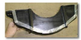
Picture 15 The dust cover should be cut along the taped line.
