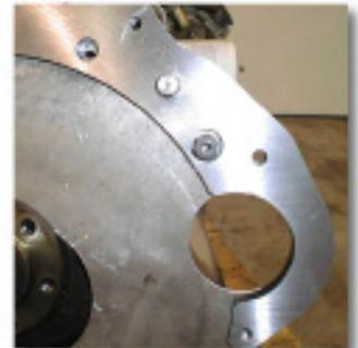
4. Your stock AMC dust cover plate and the Advance Adapters adapter plate should be installed to the back of the AMC block using the two dowel aligning bolts. A access hole should be cut in the in the dust cover to allow the bolts to be installed into the flexplate to the new aluminum adapter ring.
