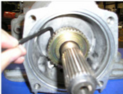
5. Tighten the 3 set screws of reluctor ring to lock it to the main output shaft. The allen wrench may need to be shortened to fit the set screws around the transmission case.
