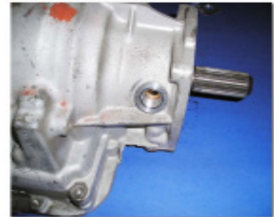
6. Test fit the bushing into the transmission housing. Make sure the bushing fits snug to the outside of the transmission. Note: You will have a small gap on the top and bottom side of this bushing, between it and the transmission.
