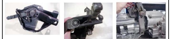
As noted on the bellhousing instruction sheet, the shifter tower of the transmission should be removed for installation. The diameter of this shifter tower is a bit larger than the Peugeot, requiring a slight floorboard modification to prevent body interference with the transmission.
