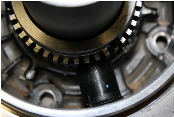
The gap between the sensor and ring must be .010"-.012" Gap
