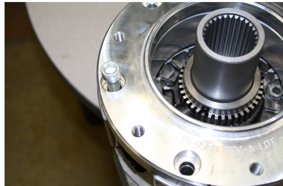
Install the 6- SHCS bolts through the two adapters and secure them to the NP205.
