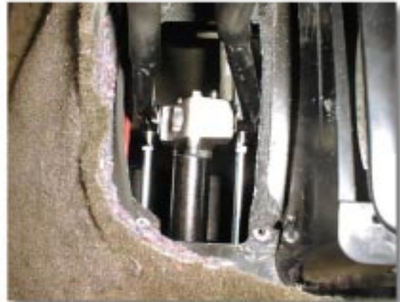
The stock hole opened up at the sides for shift lever clearance.
