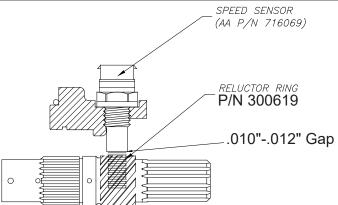
**Sensor note:** The sensor in this kit was changed in October 2005. This sensor will match up with the GM pigtail P/N 12162193 or Carquest P/N TX3A. The old sensor used in earlier kits matches up to GM pigtail P/N 12085498.
