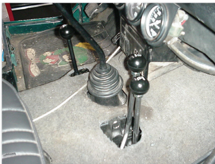
Twin sticks through modified hole in floor.
