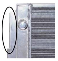
**Radiator Features:** \*1" wide core tubes, \*No Epoxies,100% TIG Welded, \*16 Fins per inch, \*Temperature Sensor Provision, \*Air Pressure Tested, \*Billet Filler Neck, \*Cross Flow Design, \*.083" Mounting Flanges.
