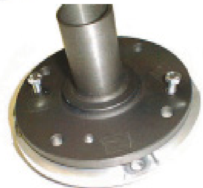
Bolt the retainers together using the two (2) 6mm bolts & Loctite 242.
