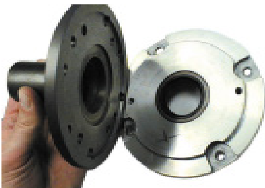
Line up holes of the modified retainer with the GM retainer holes.
