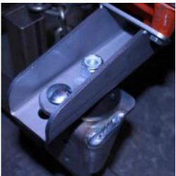
The mount can be assembled with the rubber mounts on the inner slot for a narrow frame or the outer slots for a wider frame. When the engine location is selected, tighten the carriage bolt to secures the mount location and then weld two 1/2" or more beads to secure the slide lock tab.
