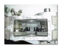
Remove the forks from the case. (Note: If you have Atlas case #1929 or earlier and have not upgraded your shifter forks, this is an ideal time to install new shift forks, P/N 301550).
