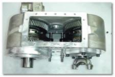
Install the cluster gear, thrust bearings, and cluster pin. Two new o-rings have been provided for the cluster pin. Be careful to make sure that the thrust washers are properly aligned between the inside of the case and cluster gear.
