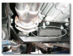
The crossmember can now be fitted to the rubber mount and the frame rails. The driver's side exhaust should fit under the crossmember and the passenger side exhaust should fit inside the crossmember. Depending on the exhaust configuration in your vehicle, you may be required to do so modifications to the exhaust for proper fit.
