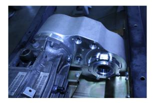
This crossmember is designed to fit the NV3550 transmission into 1966-77 Ford Broncos. This three piece mount bolts directly to the stock frame rails using the stock frame holes. The Fords frame rails are tapered from the front to the back; our crossmember mount has this same taper. When fitting the crossmember between the frame rail, a rubber mallet may be necessary to knock it into position. One of the prototype vehicles that we installed the crossmember into had some welds on
