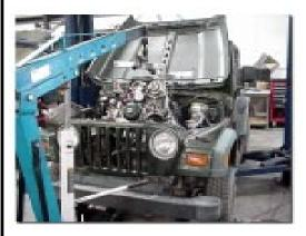
Using an approved engine hoist, lower the engine into the compartment. Pay attention to the exhaust manifolds and the radiator (removing the radiator is a good idea). The engine may not slide fully into the compartment due to firewall interferences (check the clearance on both the driver's and passenger side
