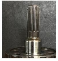
The cut shaft below shows the short splines left on the long version 6L90 output shaft.
