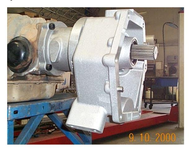
13. Fit the transmission assembly to the transfer case and secure it using the original Toyota bolts.
