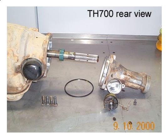
4. Cut the main output shaft 170mm from the back of the transmission as per the diagram.
