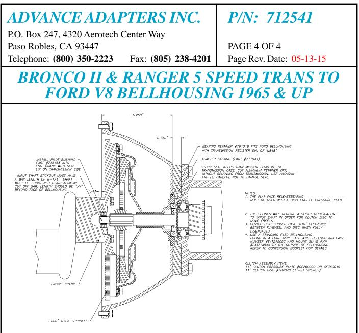
This bellhousing utilizes an external slave cylinder that works well with the Bronco II & Ranger master cylinder. This bellhousing was only used with the 164 tooth flywheel. This will cause problems with tunnel clearance, so a body lift is normally recommended. The 4 or 5 speed transmission will need slight modifications to the input shaft pilot tip, clutch splines, and stock release bearing retainer. These modifications are noted on the instruction sheet provided in this kit.
