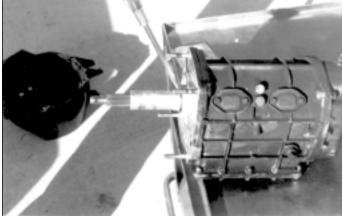
Snout will need to be cut off. The snout is only found on early model transmissions.
