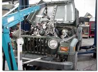
block assembly to the mount. Take a quick look around the engine and steering to make sure there are no clearance issues. You should have just enough room to fit your hand between the engine and firewall/frame.
