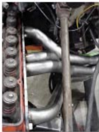
Steering clearances on 717038 headers
