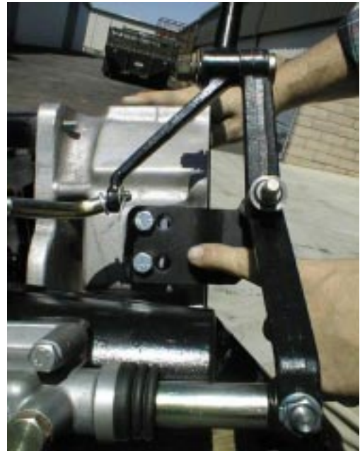
Land Cruiser transfer case linkage.
