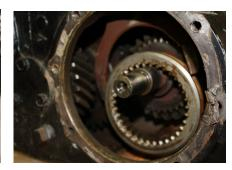
Remove the tailhousing bolts and front retainer bolts (if your transfer case has a front retainer). Shift the transfer case into 2WD high range and remove the tailhousing from the transfer case. Once the T/C output is removed, shift the T/C into low range which will release the slider. Remove the snap ring from the shaft to the bearing so the shaft and the bearing can be separated. This will allow the gear to drop downward and clear the shift fork.
