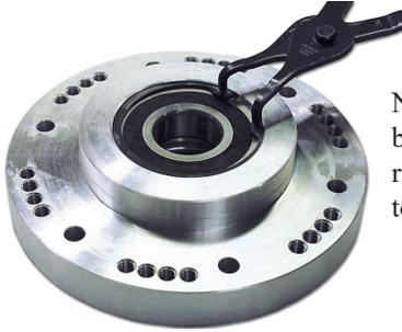
Newer Atlas T/C's use a bolt on bearing retaining retainer, this snap ring is not used. the bolts are torqued to 150 In.lbs.
