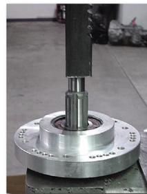
Once the gear is removed, the input shaft can also be removed. Since the input shaft is a press fit onto the front bearing, the shaft is pressed out as shown above.
