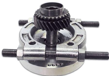
The drive gear is a light press fit onto the input shaft. It is required to be pressed off for disassembly and pressed on for assembly.
