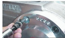
Remove the 6 Atlas input ring bolts and remove the input ring assembly from the transfer case.
