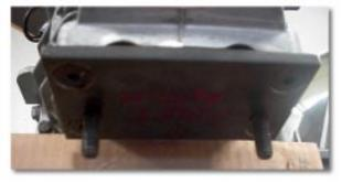
Do not over torque the 7/16 nut to stud on this plate (35 Ft-Lbs Max)
