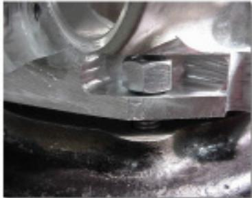
Stud bolt and nut being installed on the new tailhousing
