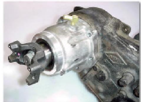
New tailhousing installed. The new bolts need to be torqued to 30ft./lbs. Turn the yoke to make sure the unit is not bound up or is not binding.
