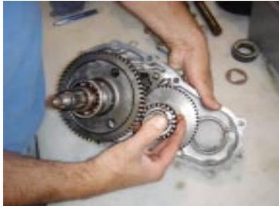
40. Slide the input gear assembly into place.
