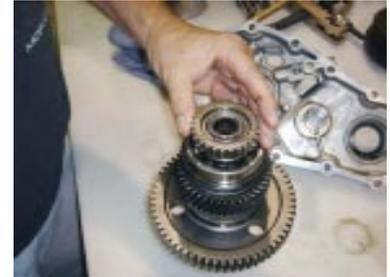
28. The input shaft/gear will now need the bearings removed and installed on the new shaft/gear. A press is usually needed to remove and install the bearings.
