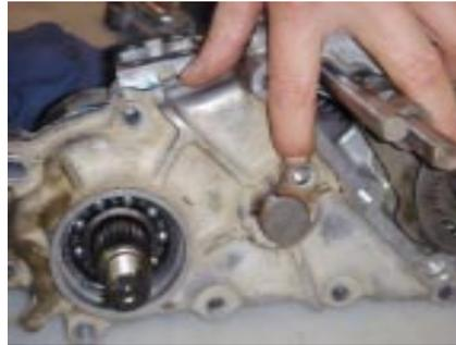
42A. You may have to twist the cluster pin in the case to install the locking tab.
