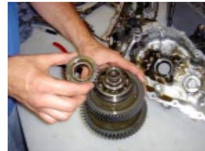
21. Using a press, press the output shaft through the bearing.
