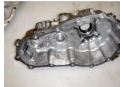
30. Inspect the front shifter housing seal and o-ring for wear.
