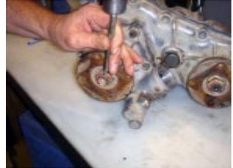
43. Reinstall the steel ball in the bottom of the case followed by the spring and the detent plug.
