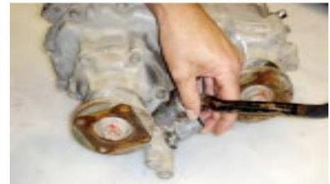
1. Drain oil from transfer case and remove the transfer case from the vehicle.
