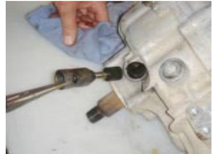
10. Remove the cluster shaft locking tab.
