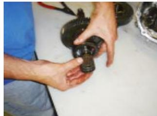
23. Under the gear is a caged needle bearing and a shifter hub that must also be removed.
