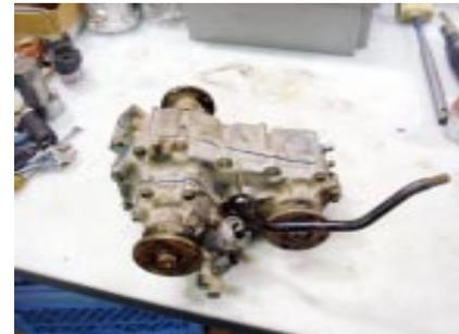
46. Install the transfer case back into the vehicle, install the shifter handle and fill with the 80/90W GL5 gear oil.
