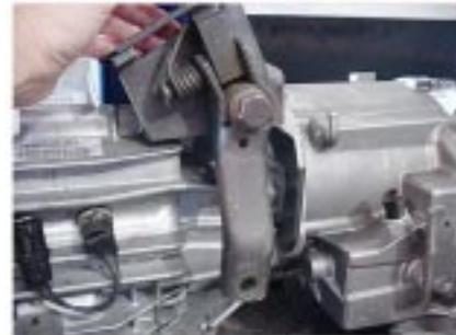
As noted on the bellhousing instruction sheet, the shifter tower of the transmission should be removed for installation. The diameter of this shifter tower is a bit larger than the Peugeot, requiring a slight floorboard modification to prevent body interference with the transmission.
